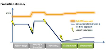
Production efficiency as a function of life cycle stages of production equipment. Several points bear the risk of a considerable drop in efficiency. The central focus of ReBORN is to counteract such losses at equipment end-of-use by enabling ist re-use and refurbishment (green bars)
