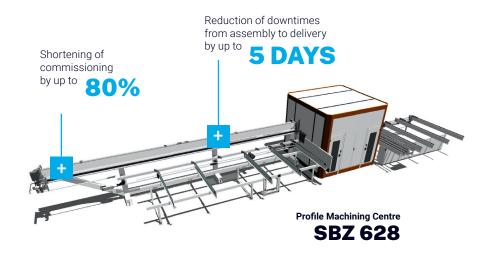
"Thanks to ISG-virtuos, we can completely commission machines with their real-time behavior with the simulation model connected to the real controller. This enables us to intercept any collisions already within the virtual commissioning and thus avoid damages and long commissioning times at the machine, which leads to enormous cost savings."
