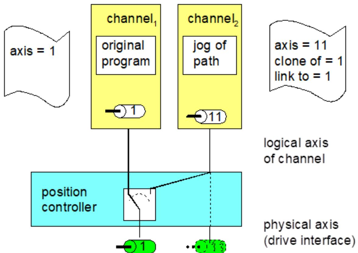
Fig. 2: Configuration of physical and logical axes
