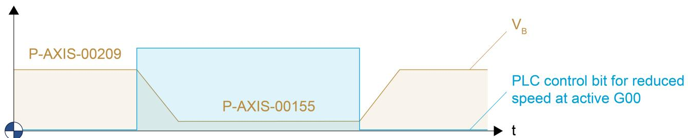
Fig. 9: Reduced maximum speed with active G00
