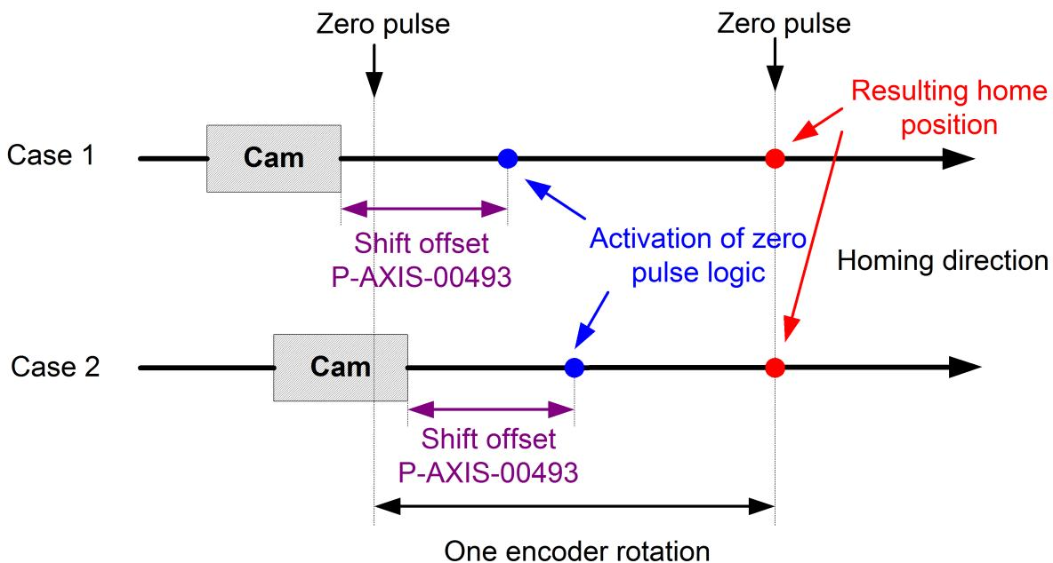
Fig. 6: Reliable detection of identical zero impulse positions
