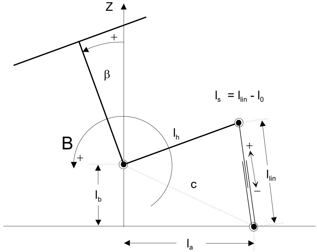
**Fig. 46: Kinematic structure of crank and linkage**
