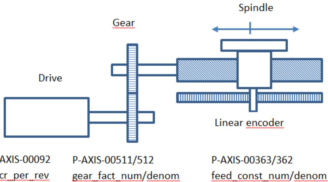
**Fig. 56: Position scaling with linear encoder**
