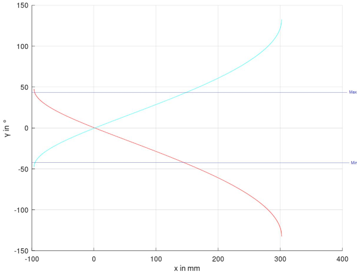
Fig. 51: Transfer function with and without angle inversion
