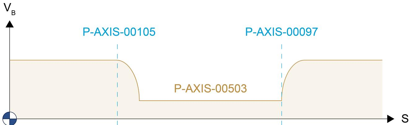
Fig. 13: Parameters of permissible axis velocities inside the second security zone
