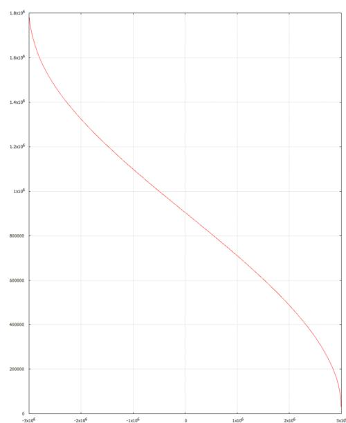
**Fig. 53: Transfer function of the symmetrical slider crank**
