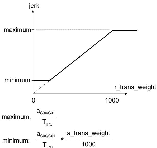
Fig. 25: Factor for jerk weighting at block transition
