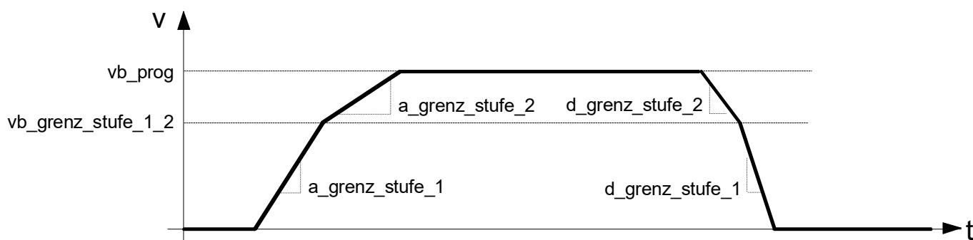
Fig. 18: Acceleration and deceleration parameters of the linear velocity profile
