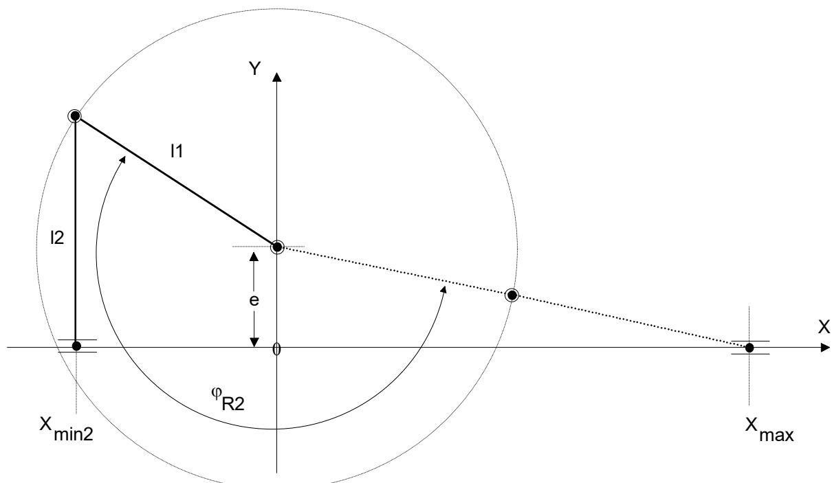
Fig. 43: Extreme positions of slider crank with eccentricity
