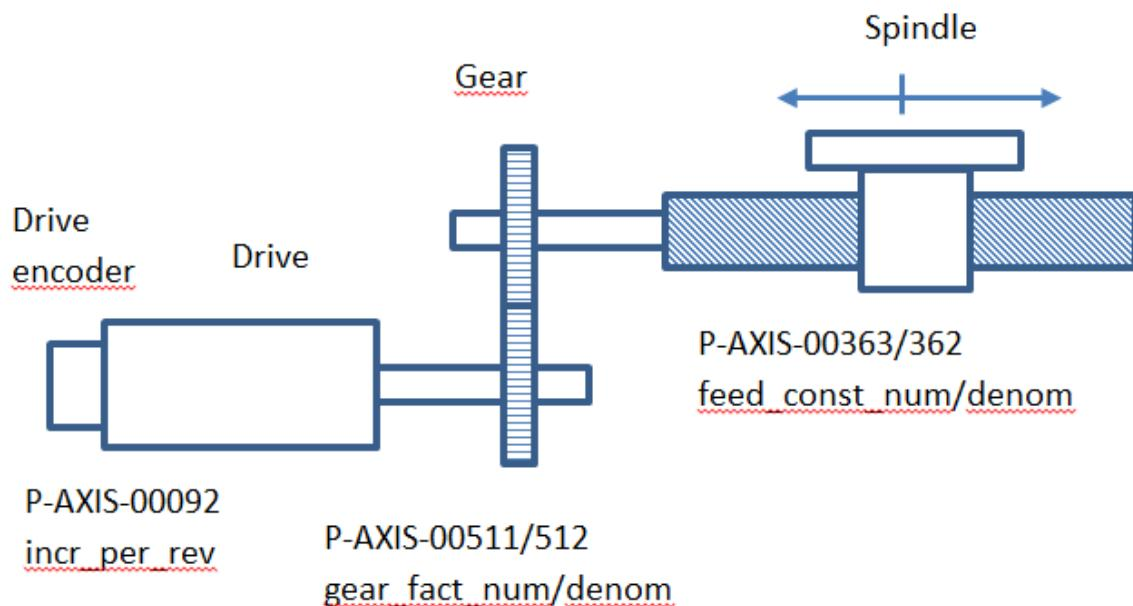
Fig. 55: Position scaling with rotary encoder
