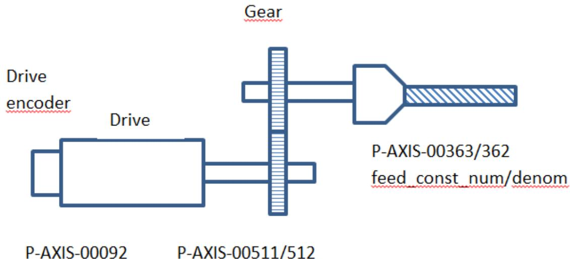
**Fig. 57: Position scaling with fitted encoder**
