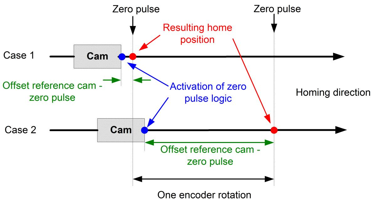
Fig. 5: Detection of different zero impulse positions possible
