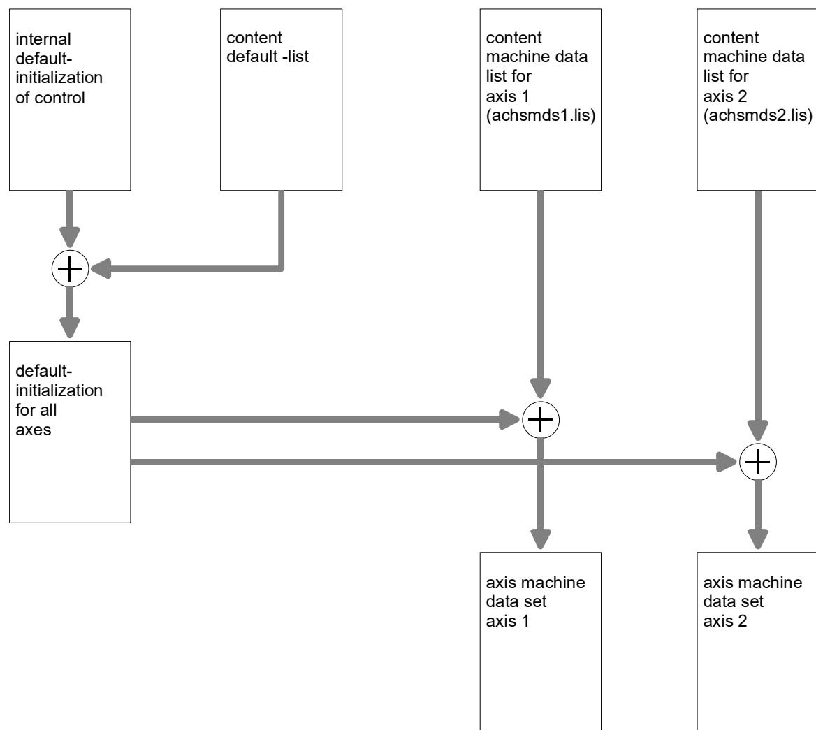
Fig. 1: List interpretation process on controller start-up
