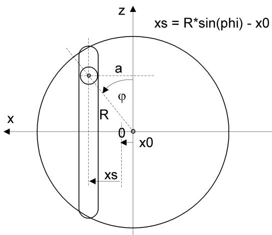
**Fig. 44: Kinematic diagram of the eccenter function**
