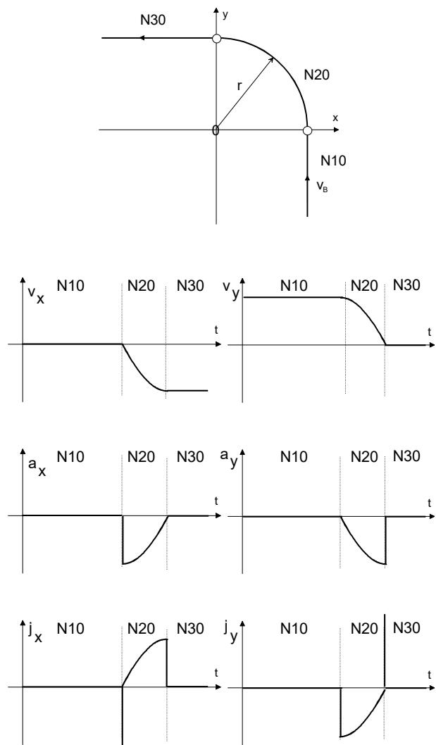
Fig. 24: Acceleration and jerk at linear-circular block transition
