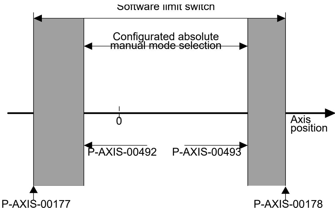
Fig. 39: Absolute motion limits in manual mode
