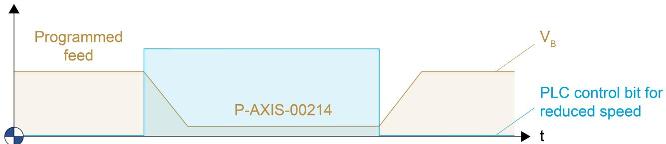
Fig. 8: Reduced maximum speed with active G01
