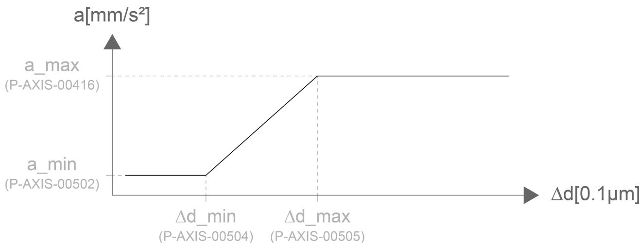
Fig. 31: Parameters for acceleration and distance error
