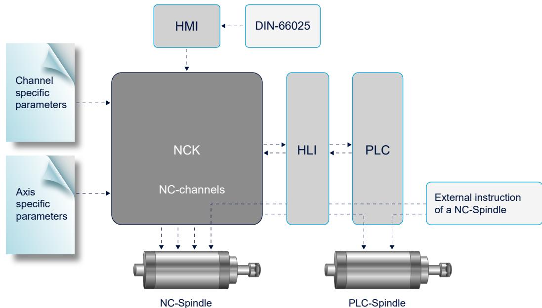
Fig. 1: Integrating spindles in the NC control topology
