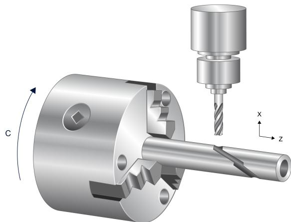
**Fig. 25: Face and lateral surface machining**
