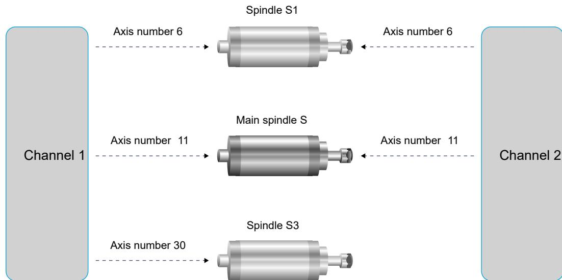
**Fig. 8: Interfacing the 3 spindles to channel 1 and channel 2**
