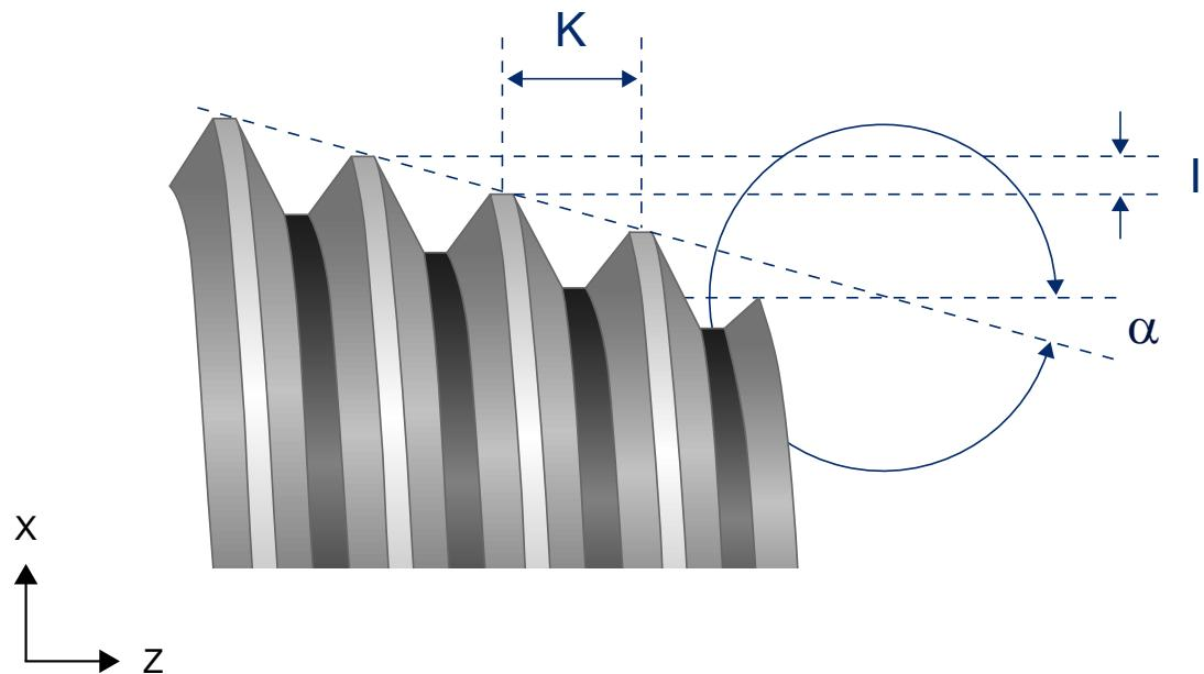
**Fig. 23: Value of thread pitch for tapered thread**
