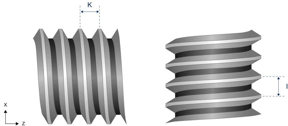
**Fig. 22: Value of thread pitch for longitudinal thread****Pitch values I, K with tapered thread**
