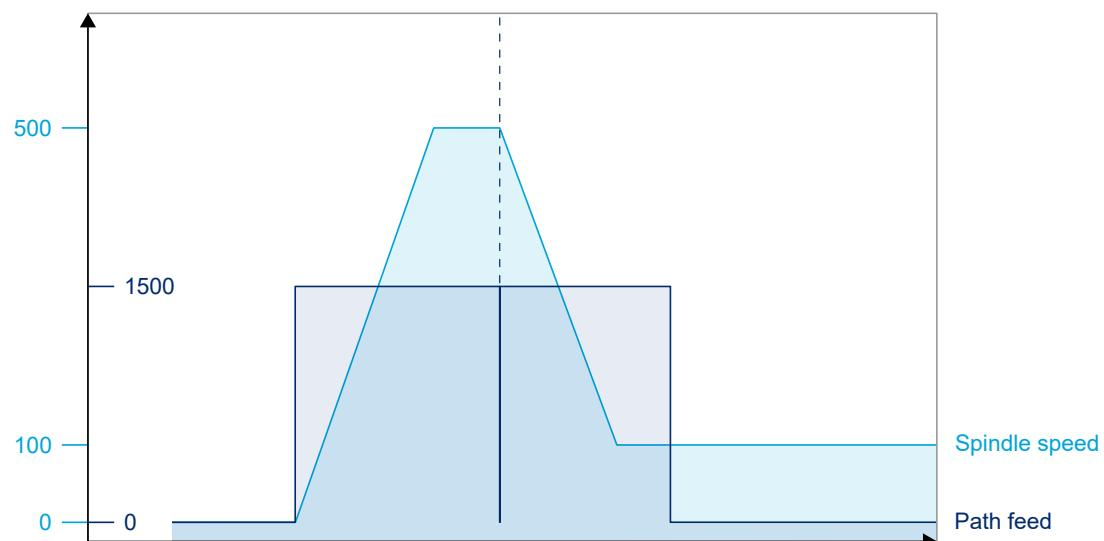
Fig. 11: Spindle not synchronised with path motion
