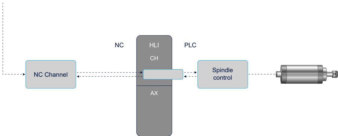
Fig. 6: Channel-specific commanding of a PLC spindle
