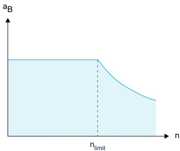
**Fig. 15: Acceleration curve as a function of speed**
