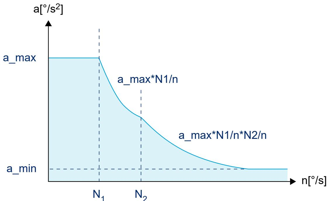
Fig. 20: Acceleration profile with asynchronous drive curve
