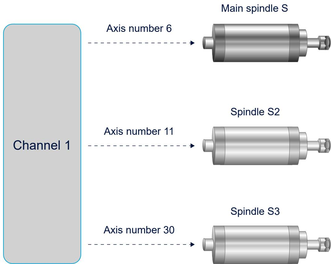
Fig. 7: Interfacing the 3 spindles to channel 1
