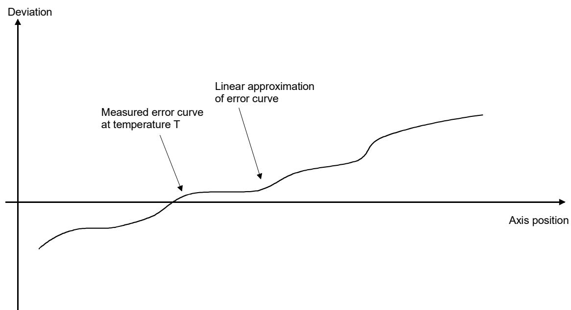
Fig. 3: Temperature-dependent falsification of the axis position
