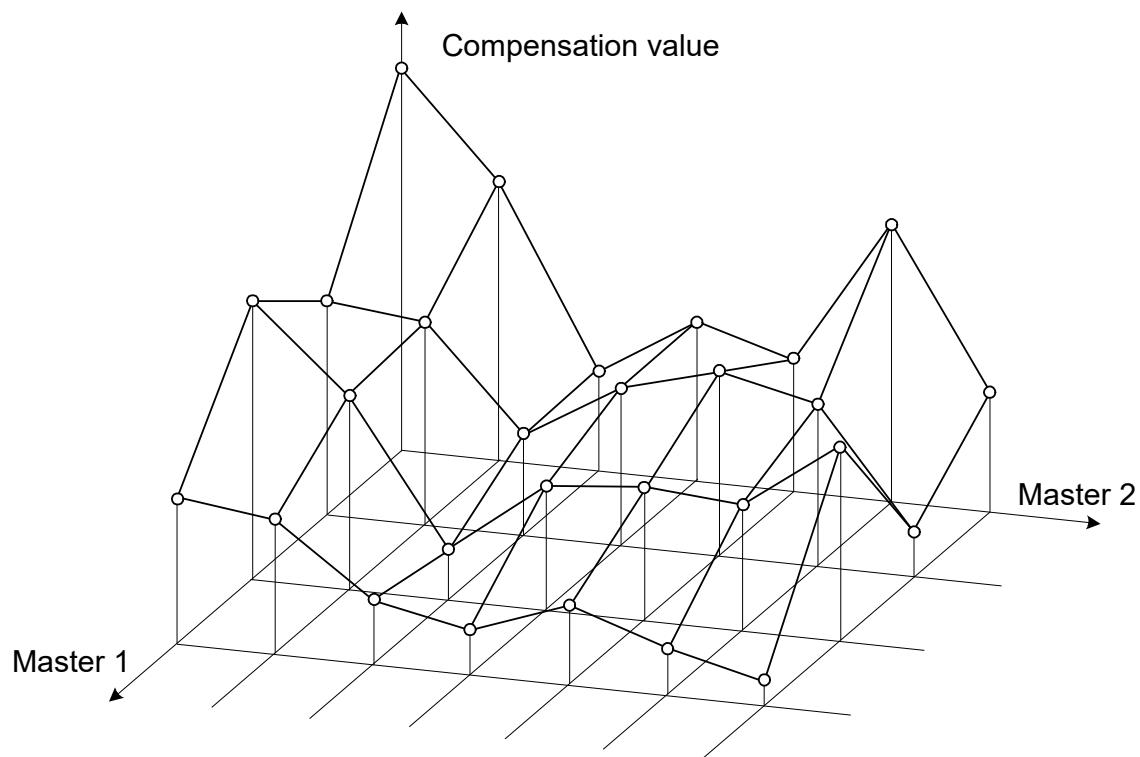
**Fig. 11: Specify compensation values at the interpolation points**
