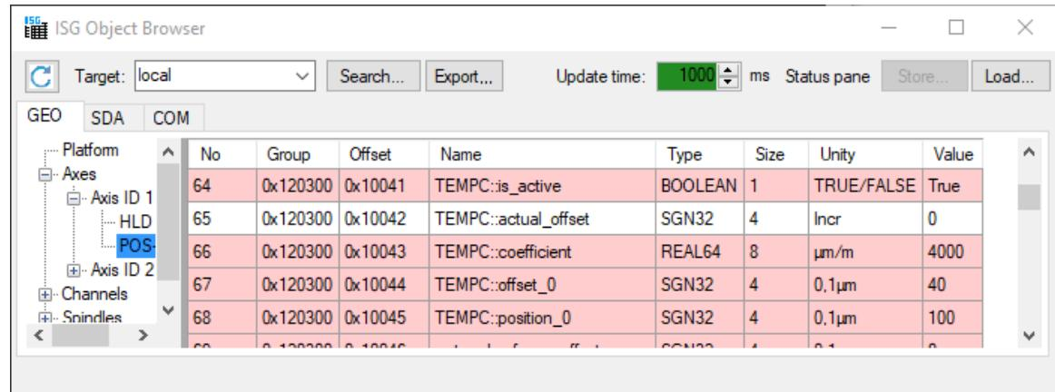
Fig. 6: Access to CNC objects of temperature compensation
