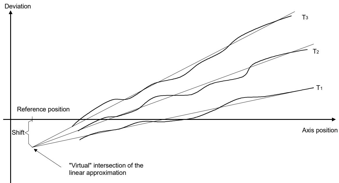
Fig. 5: Reference measurement at different temperatures
