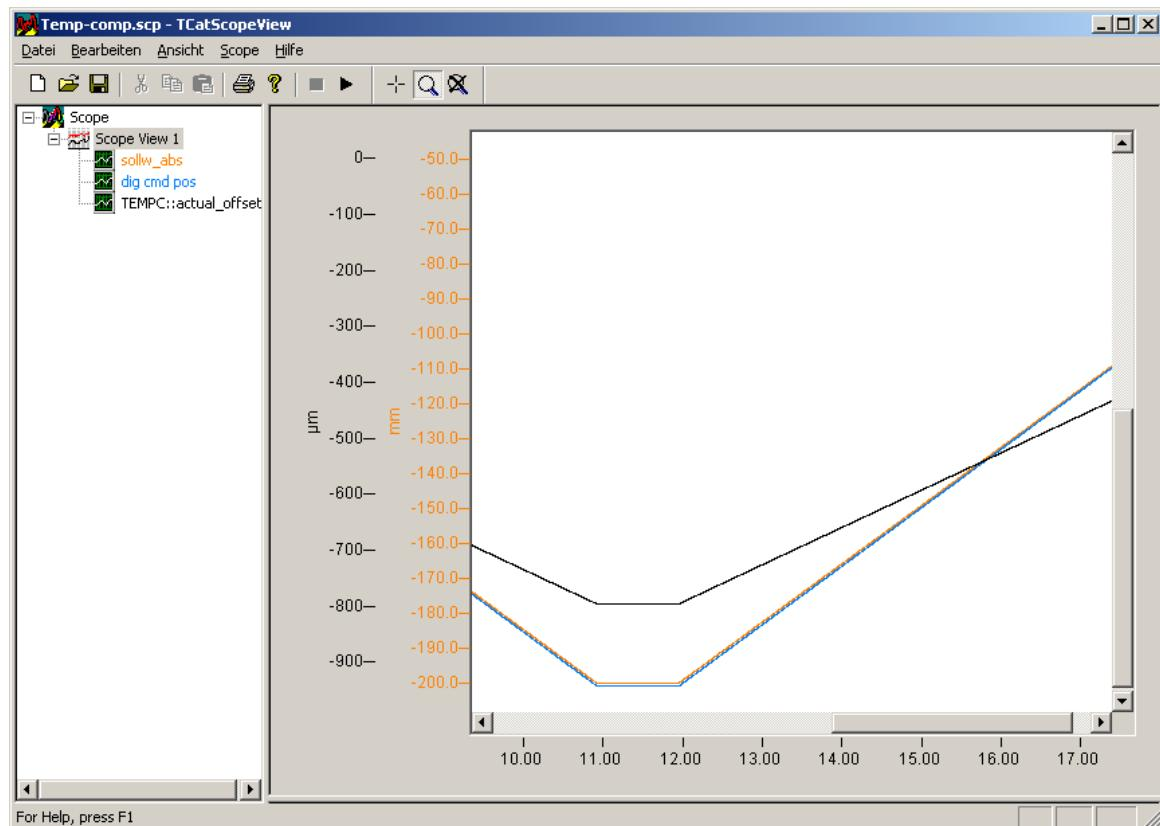
Fig. 8: Logged compensation values dependent on axis position.
