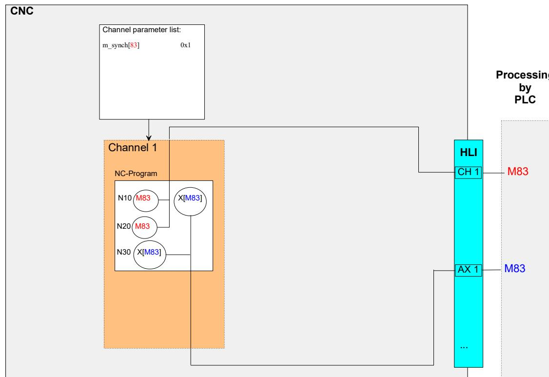
Fig. 35: Output of M83
