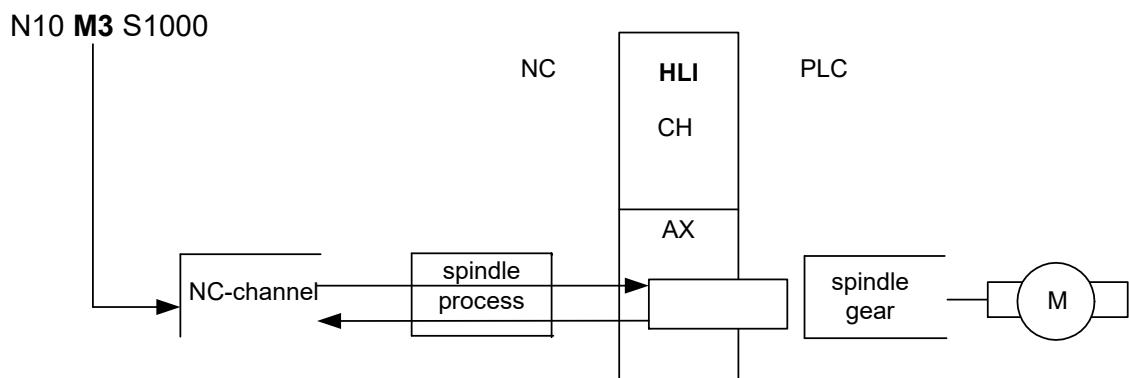
Fig. 27: CNC spindle, internally synchronised
