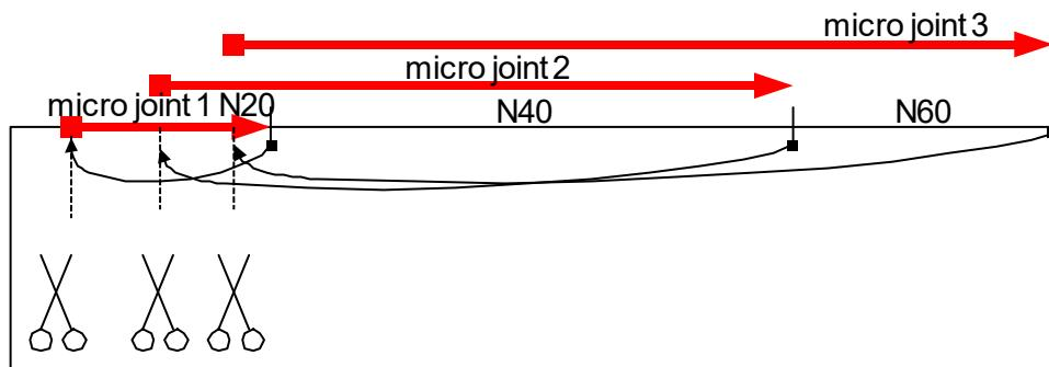
Fig. 18: Theoretical overlapping of MicroJoints in the part
