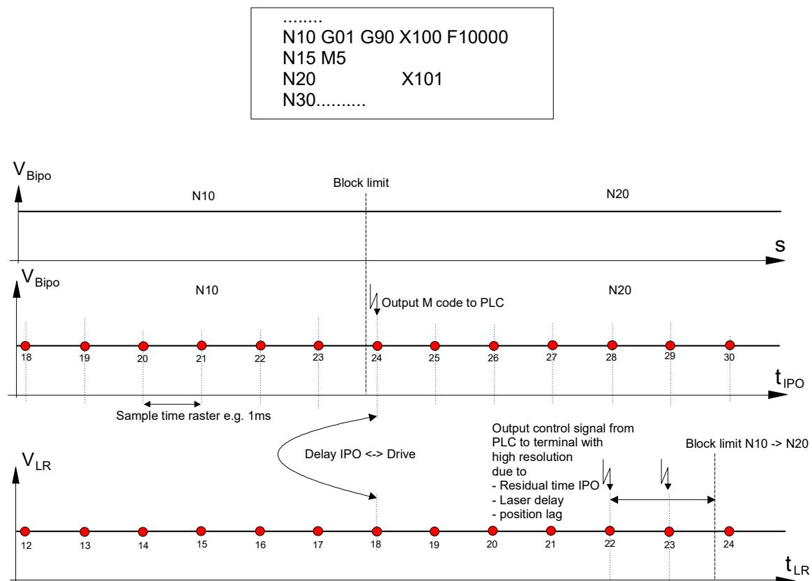
Fig. 14: Diagram of dead time compensation
