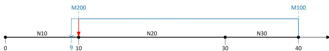
**Fig. 20: Attempted pre-output with another M/H function of the MVS\_SNS type**
