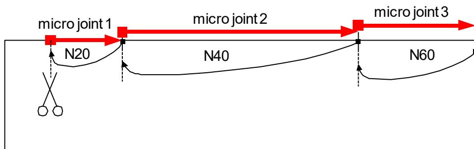
Fig. 19: Limitation of overlapping of MicroJoints in the part
