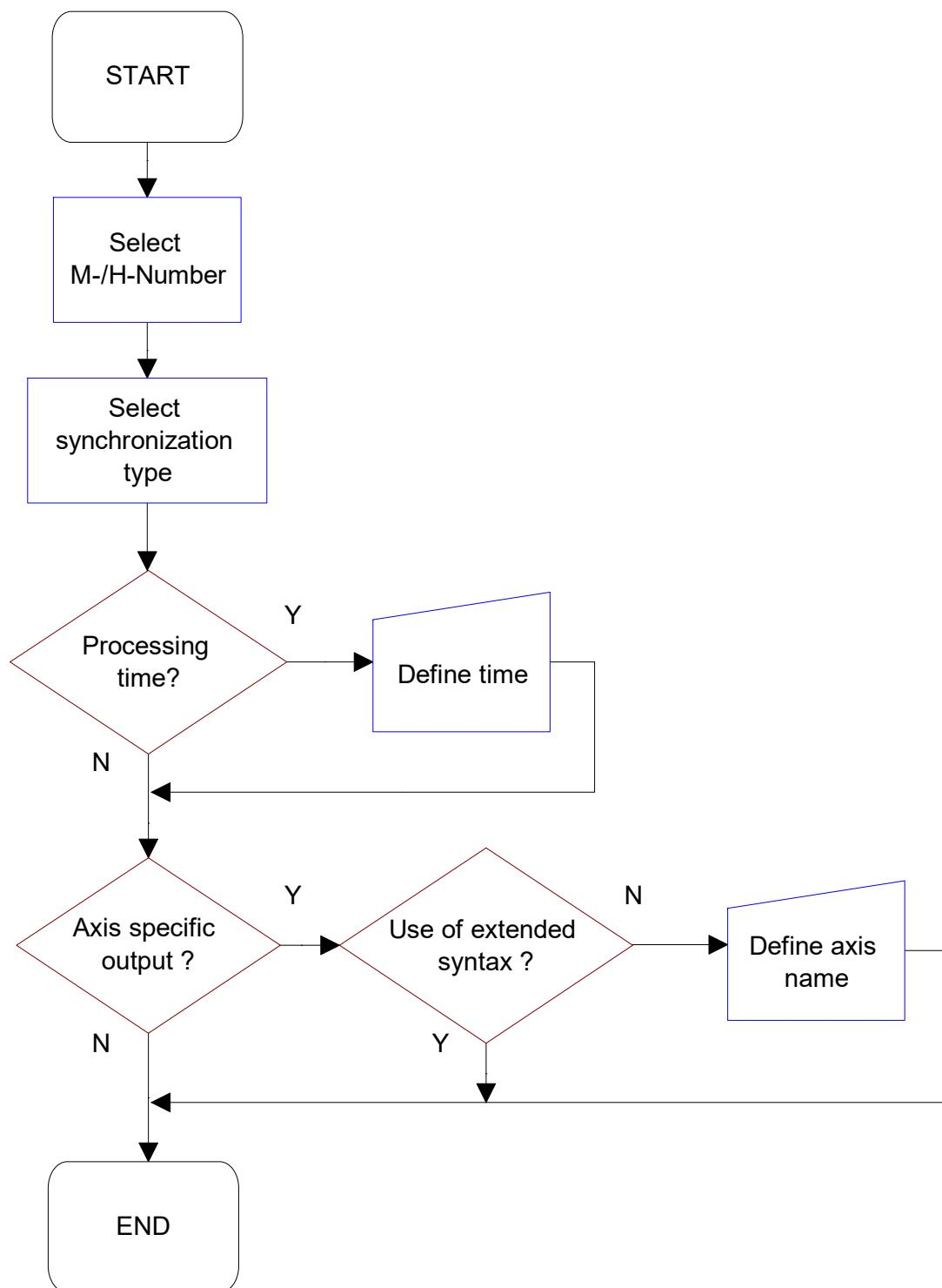
Fig. 36: Flow diagram to create an M/H function
