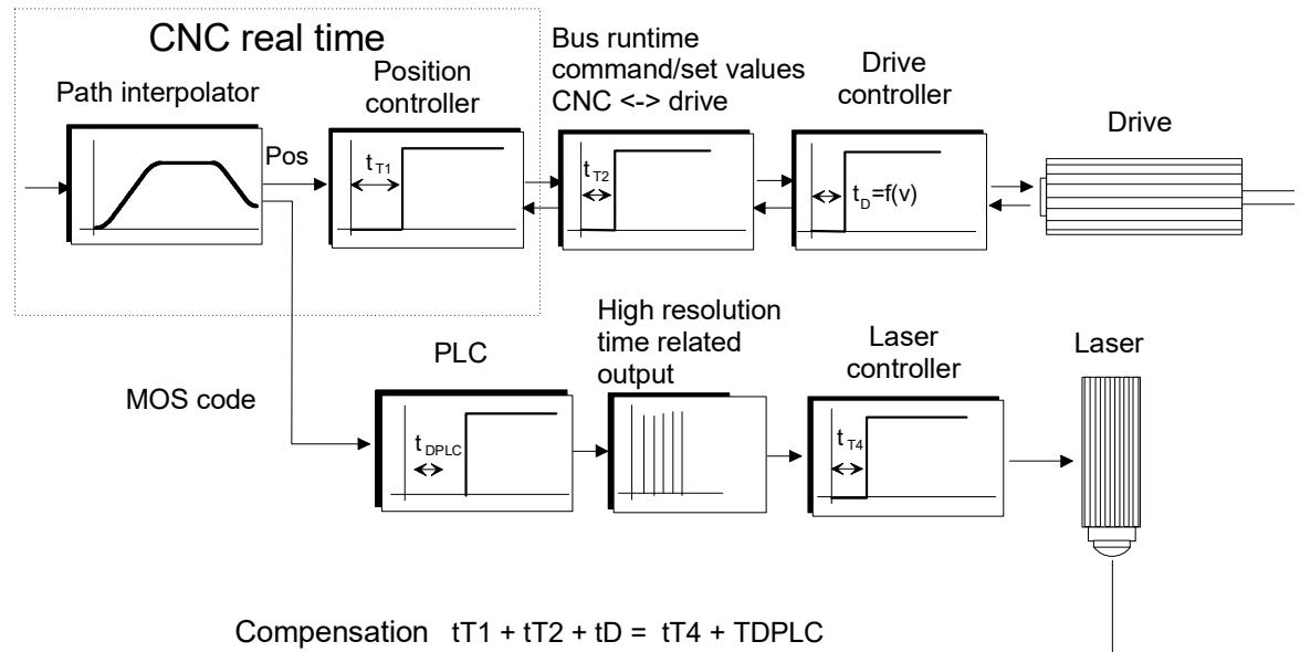
**Fig. 13: Overview of dead times in system chains**
