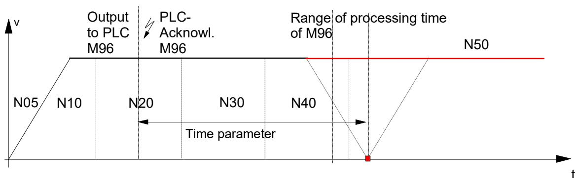
Fig. 10: Planned output time for MET\_SVS
