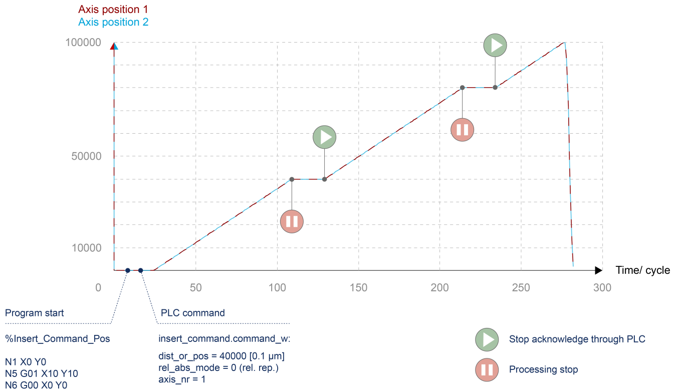
Fig. 3: Stop mark command at standstill:
