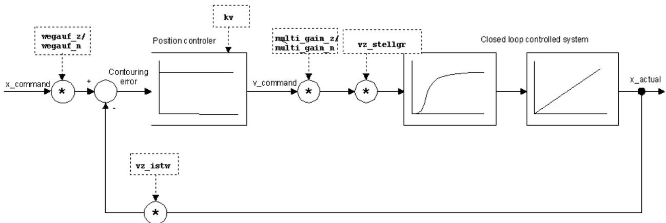
Fig. 1: Overview of the position control loop for conventional drives.
