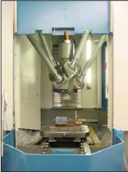
Parallel strut machine for milling purpose (HSC)
